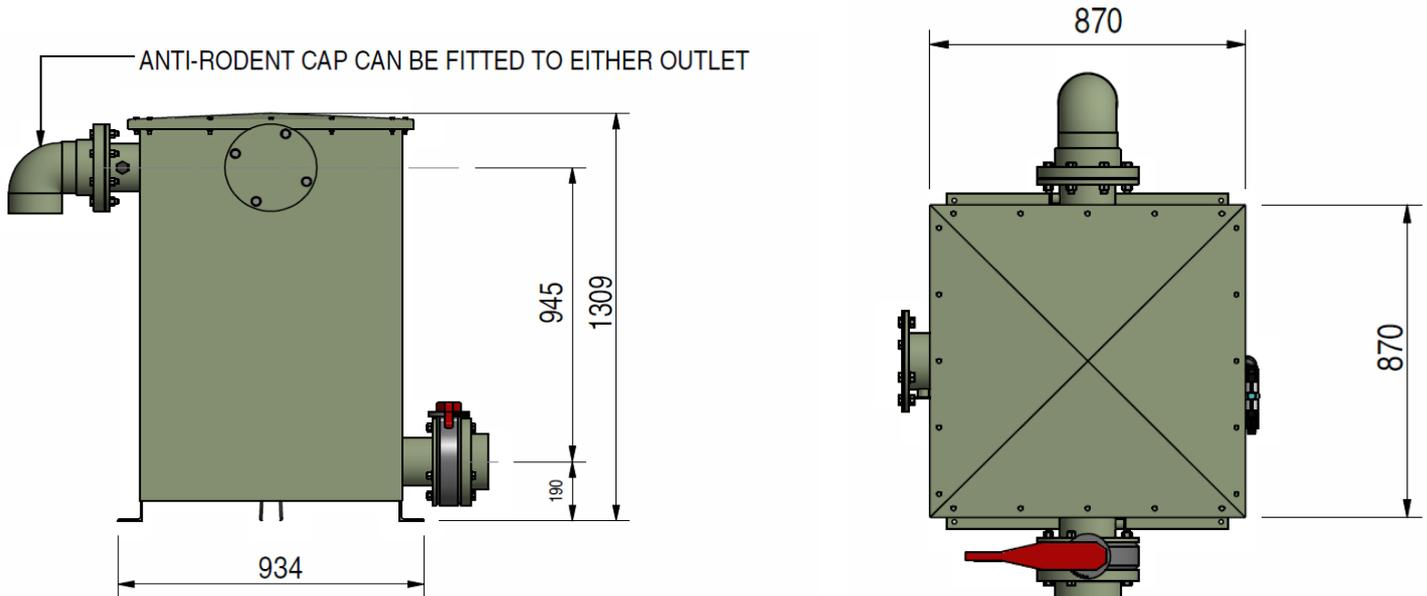
**NOTE:** CONFIRM POSITION OF INLET AND OUTLET FLANGES AS THESE CAN BE POSITIONED TO SUIT SITE REQUIREMENTS
